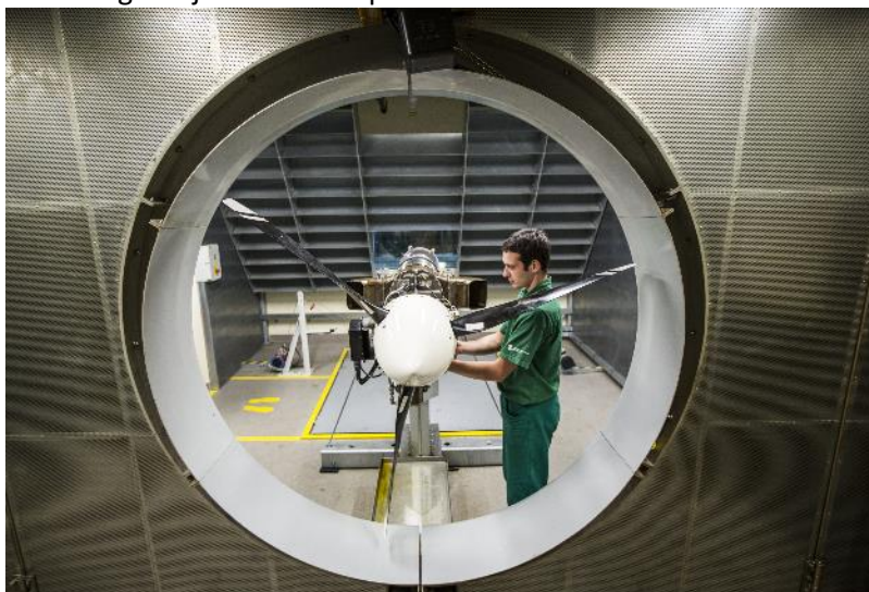
Fig. Testing the TJ 1P100 turbo-prop engine in the test laboratory at the aviation division of PBS
